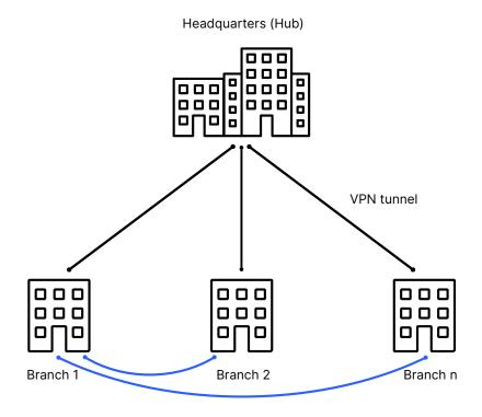
Figure 3: Site networking via Advanced Mesh VPN
