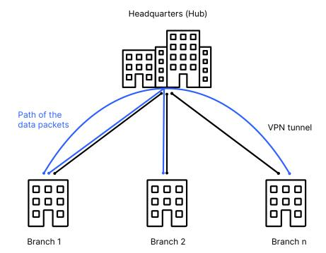
Figure 2: Data exchange between branches with classic site networking (hub & spoke)
